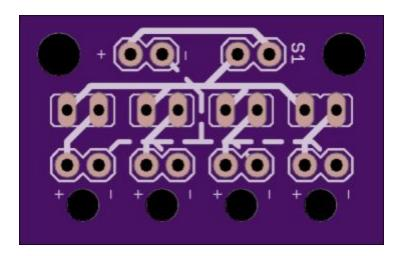
The thick solid lines indicate the flow of electricity. From the above image, you can see that it starts from the battery's +, moves to the S1 switch, and then is distributed across the middle pads (from this orientation, the left pad of each pair). It then goes to each of the output + pads.
