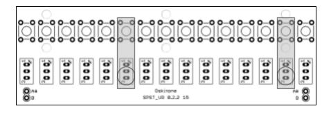
To short the pads, apply generous solder to each, then solder the middle until the two connect. You can do this on either side of the PCR
